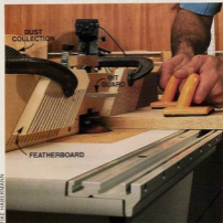
Photo 1 Featherboards, bit guards and dust collection allow you to safely do things with a router table that would be impossible with the router alone.
