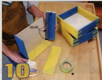
10 Hold the parts of smaller drawers together with masking tape. Be sure the boxes are square before setting them aside to dry.
