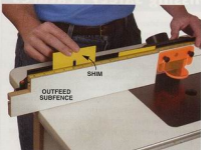
Photo 6 A subfence allows you to offset the outfeed fence with shims for edge jointing. Some manufacturers include shims, but you can easily make your own from paper, cardboard or plastic laminate.
