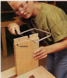
FIG. F Haunched Apron Tenons
