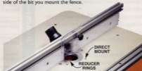
Photo 12 Direct mounting the router to the top creates an uninterrupted surface free of catch points caused by a mounting plate. Direct mounting also requires a much smaller hole, which results in a stronger top. On the downside, it's a hassle to remove the router for hand-held work.
