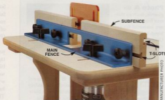
Photo 7 T-slots in the subfence work great, but in order to make your own subfence, you'll need to purchase a specialized router bit ($25). We prefer the easy-to-make subfence shown in Photos 4 and 5.
