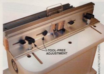
Photo 8 Tool-free adjustment knobs are the only way to go. The last thing you need to keep track of is another screwdriver or Allen wrench.
