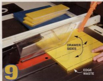
9 Rip the drawer parts to final width and then saw or rout a dado for the drawer bottoms.
