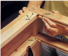
16 WOODEN SPLINES ALIGN THE RUNNERS AND RAILS PERFECTLY, just like a tongue-and-groove joint.
