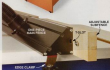
Photo 4 Here's what to look for in a router-table fence: Edge clamps allow you to position the fence anywhere on the table. A one-piece main fence doesn't have the alignment hassles of a two-piece fence. T-slots make convenient attachment points for subfences and accessories.
