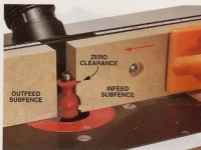
Photo 5 An adjustable sacrificial subfence is a must-have feature. The subfence allows you to adjust the fence opening to accommodate any sized bit. With the main fence secure, you can even push the infed fence into a spinning bit and create a zero-clearance opening to eliminate chip-out.
